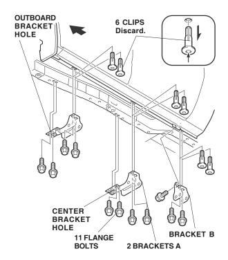
7. Install two brackets A and one bracket B to the body using 11 flange bolts. Thread the flange bolts in about 3 to 4 threads. When installing brackets A, use the outboard bracket holes for the front bracket, and the center bracket holes for the center bracket. 8. Install the side step to the brackets using 12 flange bolts and 12 flange nuts. Thread the nuts on about 3 to 4 threads.
