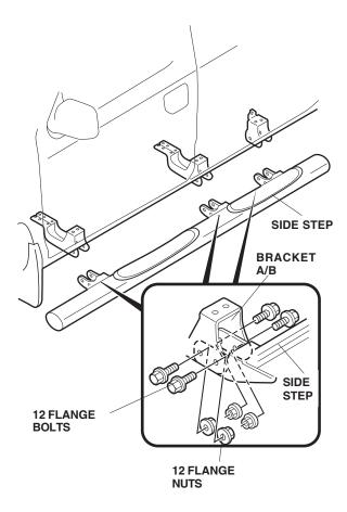
9. Adjust the location of the left side step so there is even clearance between the side step and body, then tighten the flange bolts you installed in step 7. Torque 10 flange bolts to 27 N·m (20 lbf·ft), and the one remaining flange bolt to 7 N·m (5 lbf·ft) as shown.
