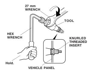
5. Remove the tool from the knurled threaded insert by turning the hex wrench counterclockwise.
